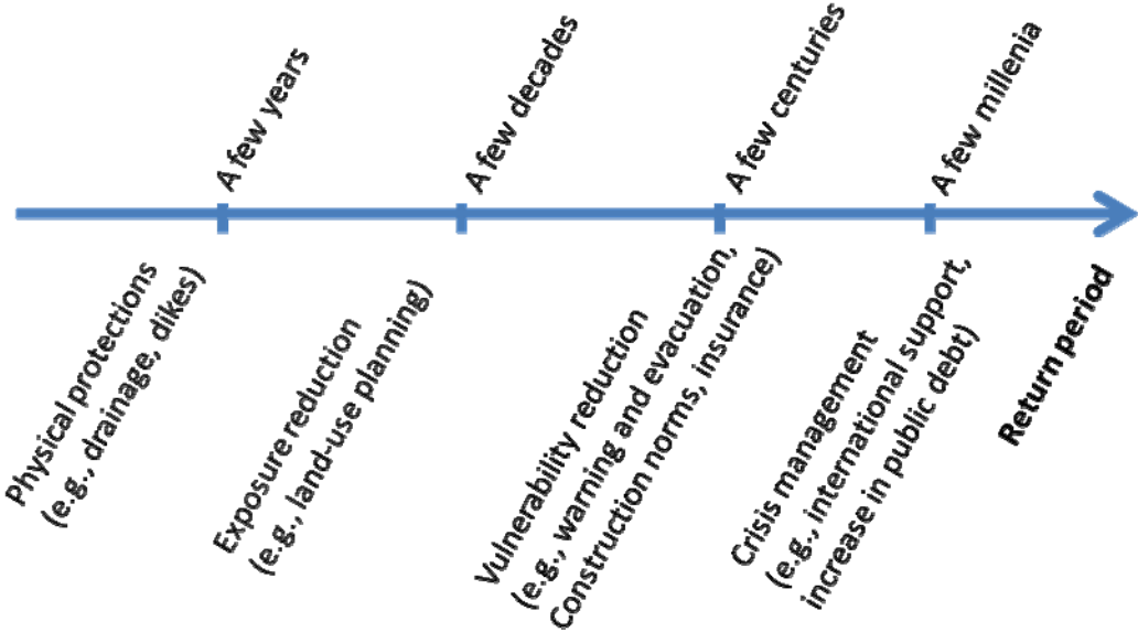
Figure 4: An example of risk-management policy mix, in which physical protections avoid frequent events; land-use planning limit population and asset exposure if protections are overtopped; early warning, evacuation, insurance reduce vulnerability, increase resilience and help affected regions rebound; and finally crisis management and international solidarity help cope with the largest events.
